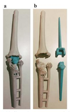
**Fig. 4** Models of bone and components were created using a 3D printer. a) Components were inserted and b) removed.
