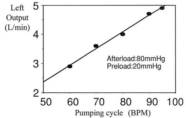
**Fig. 9.** Performance of the left pump in the second step of the study using DC actuator (100W, 24V). Stroke volume is 52 ml. Calculated diaphragm displacement is 12mm.
