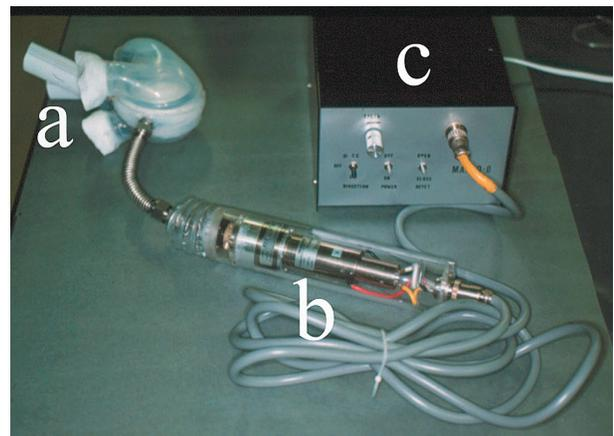
**Fig. 7.** A whole view of the assembled system. Character "a", "b", "c" indicate blood pump, actuator, and controller and power supply, respectively. The blood pump is coupled with actuator with connecting wire and connector. The actuator is also hooked up to the controller and power supply via a shield line.
