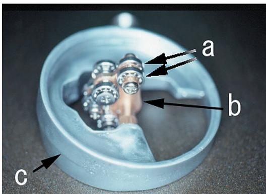
**Fig. 4.** A supporting frame and the assembled cam are shown in ready-to-go condition. Character "a" indicates bearings assembled into cam plate (b). Character "c" indicates supporting frame.
