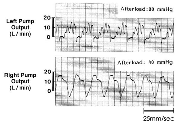
**Fig. 11.** Traces of the left and right flow. Systolic duration per cycle is calculated 68% during the measurement. Flutter phenomena is seen in the left output.
