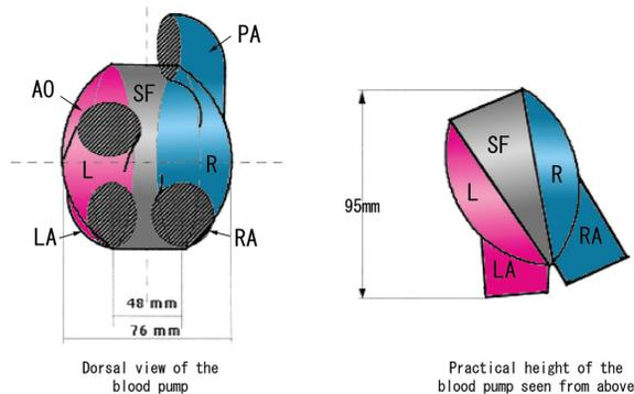
**Fig. 3.** Ideal measurement made on a design specification of the blood pump is shown. Practical margin of error is not considered which may appears in a course of fabrication. Characters in the figure indicate each pump sites as follows: AO: aortic port, LA: left atrial port, PA: pulmonary arterial port, RA: right atrial port, L: left blood chamber housing, R: right blood chamber housing, SF: supporting frame.
