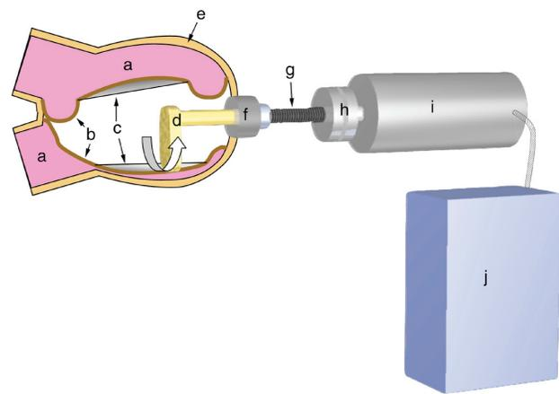
**Fig. 1.** Basic concept of the STAH system. Each character in the figure indicate system parts as follows; a: left or right blood chamber, b: left or right diaphragm, c: left or right pusher plate, d: cam, e: pump housing, f: connector, g: connecting wire, h: coupler, i: actuator, j: controller and power supply. A unit of the blood pump is consisted from a to f, and a unit of driving unit is from g to j, respectively. A big blank arrow shows an ideal direction of cam rotation.
