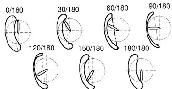
**Fig. 2.** Schematic drawing of relationship between the cam and pump diaphragm at each angle of the cam. Angles are shown by each degree per 180 degrees.
