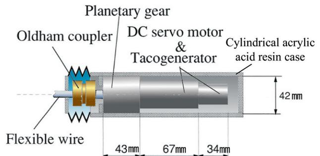
**Fig. 5.** Mechanical configuration of the actuator. Planetary gear, DC servomotor, and taco generator are coupled in production process. Each height is 43, 67, and 34mm, respectively as shown in the figure. Planetary gear brings maximum diameter by 42mm. These units are installed into a cylindrical acrylic acid resin case with 2mm thickness.
