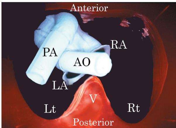
**Fig. 8.** The blood pump installed in the chest cavity model. AO: aortic port, LA: left atrial port, PA: pulmonary arterial port, RA: right atrial port, Lt: left chest cavity, Rt: right chest cavity, Anterior: Ventral side of the humane body, Posterior: Dorsal side of the humane body, V: Vertebra.
