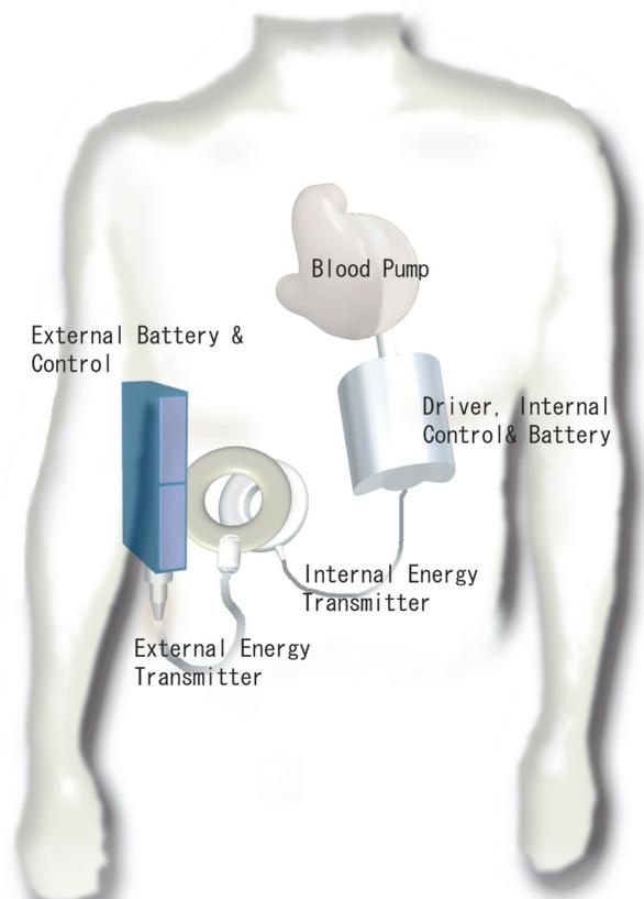
Fig. 12. Outline of the final system of the STAH.
