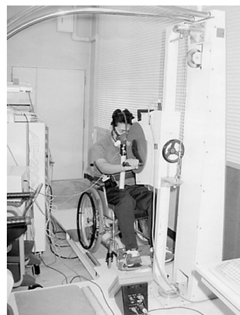
Fig. 1. The modified arm ergometer for the wheelchair user. The ergometer can be easily adjusted at variable height in relation to the wheelchair seating position of the subject.
